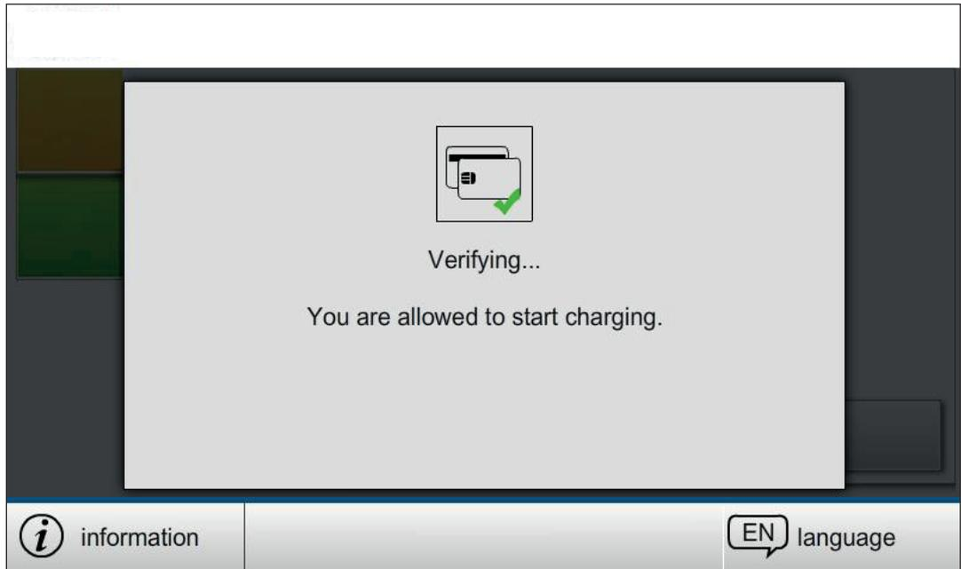
5. Preparing: the charger and the vehicle perform a handshake and the necessary safety tests. Charging will start automatically when successful.
