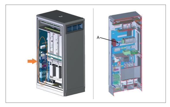
1. Route the CAN cable(s) to the terminal block (A). Refer to the figure for the preferred cable route inside the cabinet.
