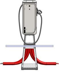
3. Concrete mount See paragraph 3.4 Install base frame on the floor or 3.5 Install base frame on the floor with chemical anchors for civil work and mechanical installation on the floor. After that see paragraph 3.6 Install the column on the base frame
