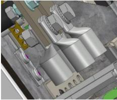
The earth connection is just below the DC connections:
