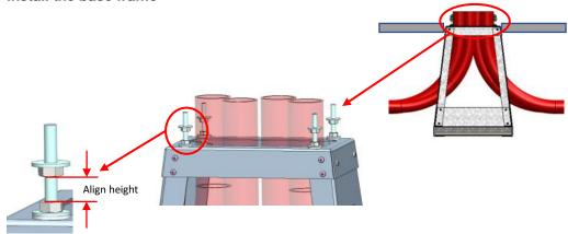
1. Install the threated rods with washers and nuts onto the foundation.
