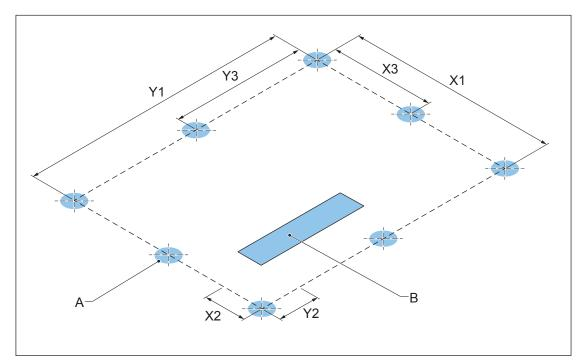
A Holes to install the fasteners of the EVSE B Hole for the cables
