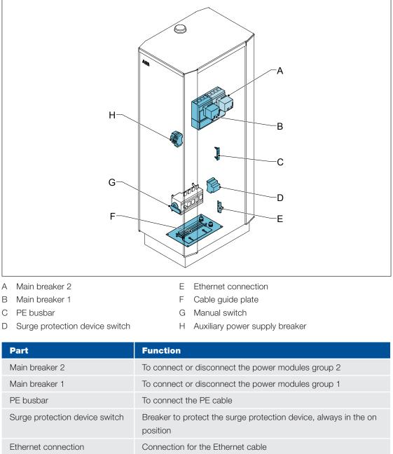
Cable guide plate Plate with openings for the AC input cable and the Ethernet cable Manual switch To connect or disconnect the AC power input To connect or disconnect the AC power input to or from the
